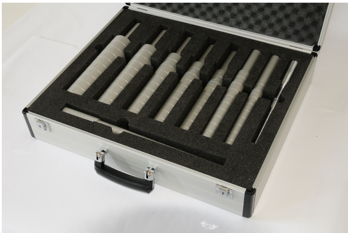
Pipe insulation thickness dorn set
